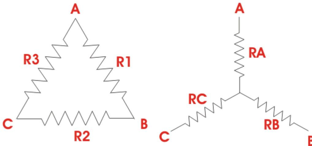
Consider a delta system that's three corner points are A, B and C as shown in the figure.
